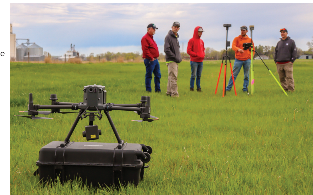
JEO Consulting used a drone to record ground elevations as part of the Lower Loup NRD's Sargent Flood Resiliency Project.
