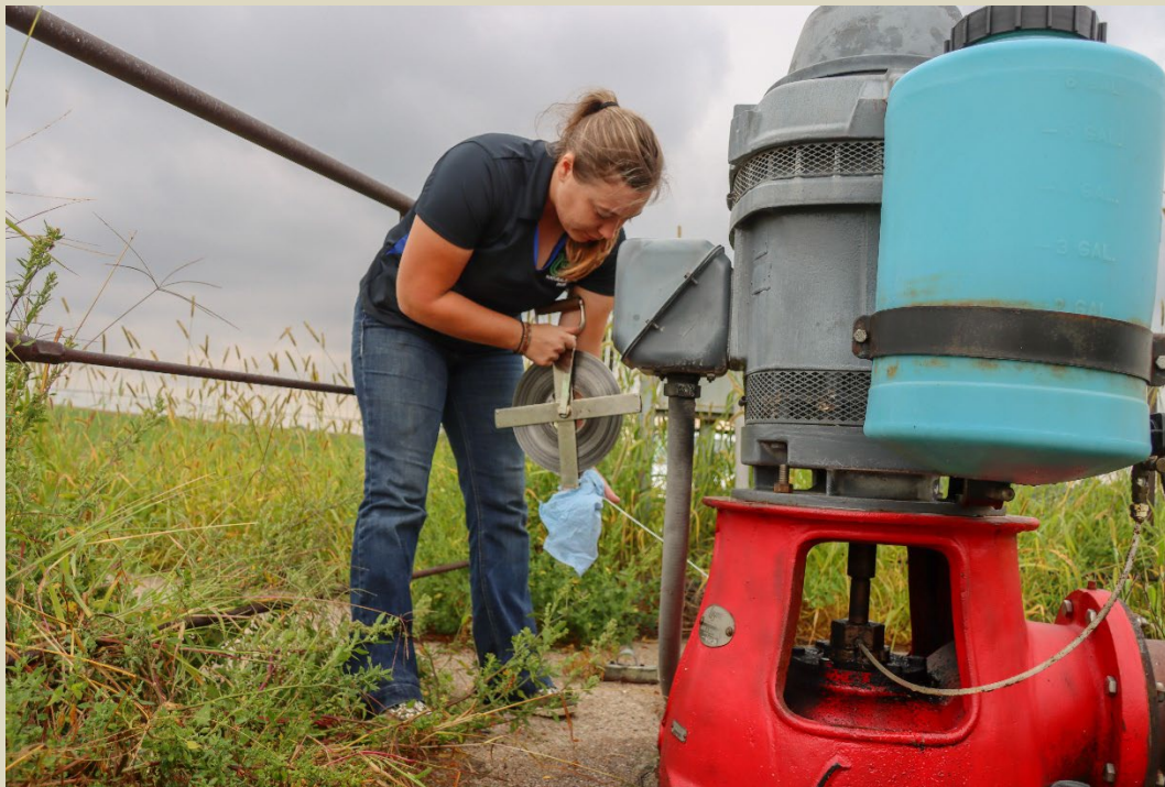
Field Staff Collecting Static Water Level
