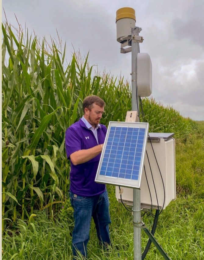
LLNRD field staff downloading data from soil moisture station near Cedar Rapids
